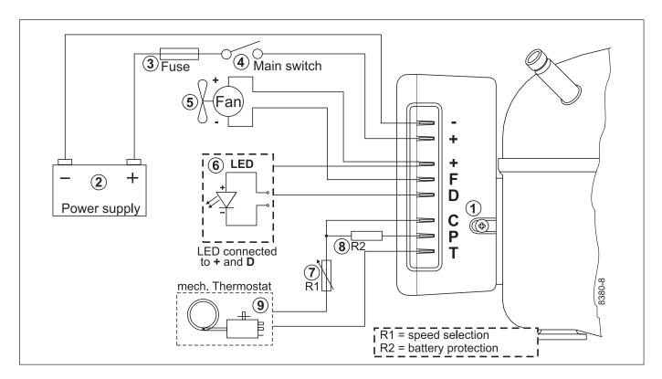
The electronic unit is a dual voltage device. This means that the same unit can be used in both 12V and 24V power supply systems. Maximum voltage is 17V for a 12V system and 31.5V for a 24V power supply system. Max. ambient temperature is 45°C.
